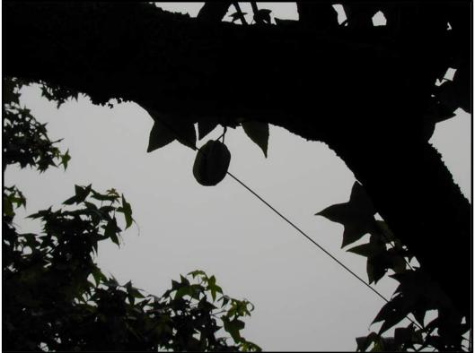
The standard strain insulator hangs from a branch. The beverage wire lays across the insulator webbing, fully floating. Only the hanging wire wraps the web.
